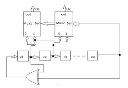
Figure 8. Bit Swapping LFSR
